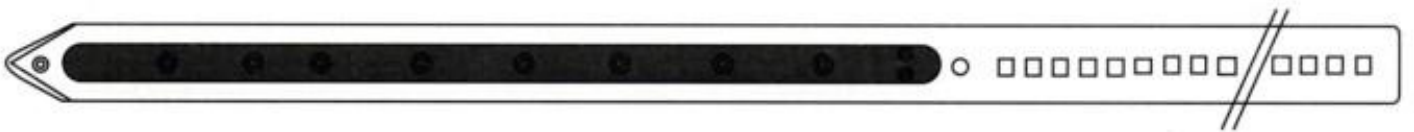
ISHIKAWA RAPIER TAPE 1001 FOR CARBON SUPPORT WIDTH 30 mm. RIGHT
